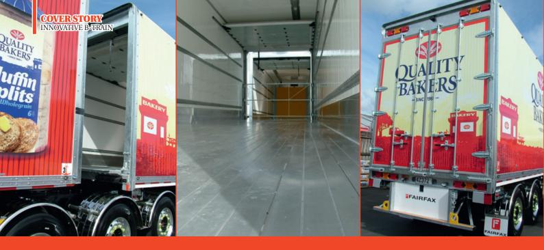
**Above left:** Rear of front trailer and front of rear trailer have roller doors to allow access between both for loading. **Above centre:** A view looking forward from the back of the rear trailer. Trailers have forklift-rated alloy floors. **Above right:** Trailer is fitted with reversing camera (black box at top centre) and Wabco Tailguard for added safety. **Bottom:** B-train runs SAF Intradisc axles.
