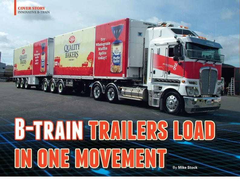
ANTERBURY TRANSPORT OPERATOR KERRY INNS' new B-train has trailers that can be driven together and loaded as one, using a Phantom loader that drives through the unit.
